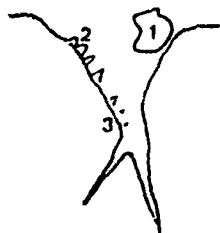
Figure 8. Pore structure (schematic). 1, Colloid or polymeric molecule; 2, Large adsorbed molecules (e.g., detergents, dyes, humic compounds); 3, Small adsorbed molecules (e.g., solvents, iodine) (Masschelein 1992).
